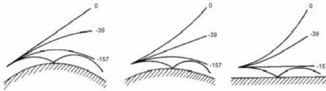
Fig. 5.8. Representation of horizontal trajectories with respect to the refractivity gradient for different representations: real Earth, effective Earth's radius equal to 4/3a , flat Earth
