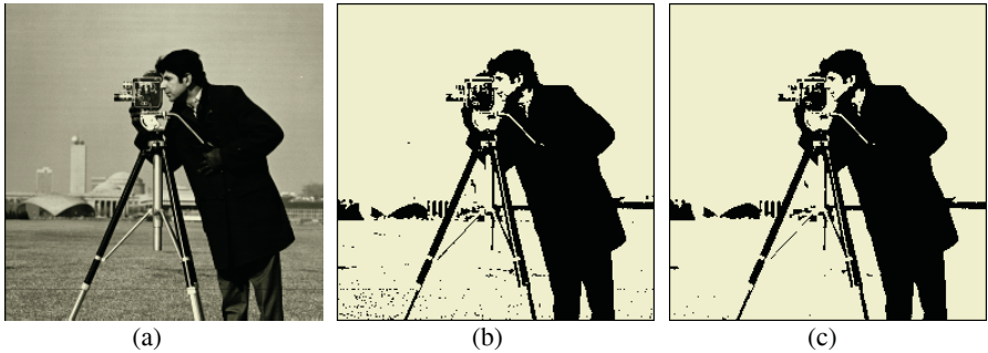
Fig. 3. Comparison of segmentation results on a real standard image named cameraman . (a) The original image. (b) FCM result. (c) PFCM result
