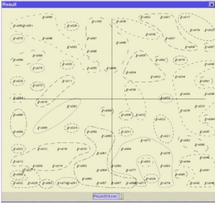
Fig. 6. Clusters generated in SOFM with a sole image attribute from line segments
