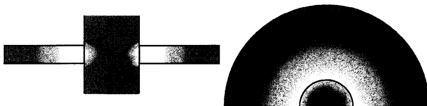
Fig. 9.2. Circular cylindrical resonator, E_{010} mode, resonance frequency 2.5 GHz, resonator is filled with dielectric material except in the aperture, view of halve of the resonator, chimney, left: magnitude of E-type in a cross section, right: magnitude in a middle slice of the resonator, white high magnitude, black low magnitude
