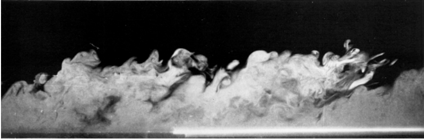
Figure 8.26. Flow visualization of a boundary layer in subsonic flow at Re_\theta \approx 4000 , obtained by seeding the flow with a fog of oil droplets, and illuminating the flow with a planar laser sheet (Falco, 1977). Flow is from left to right. (Copyright 1977, AIP. Reprinted with permission.)
