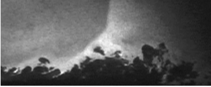
Figure 10.26. Filtered Rayleigh scattering image of a sharp-fin interaction at Mach 8, with Re_\theta = 2400 . The view is in a plane aligned with the incoming flow direction. Incoming flow is from left to right. Within the interaction, the flow is out of the page at approximately 16^\circ . (From Bookey et al. (2005a), with the authors' permission.)
