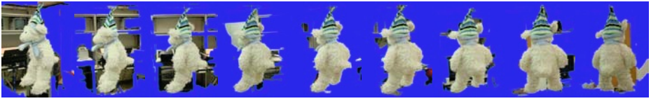
Fig. 2. Silhouette estimations in the first 9 steps: Note that they are over-estimations. The new estimations are computed based on the previous estimations
