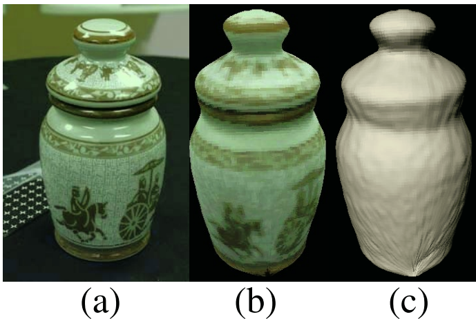
Fig. 4. Result of Silhouette Carving Algorithm: (a) One of input images, (b) Result with color, (c) Result without color
