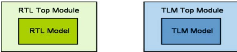
Figure 5-14. Separate Top Modules as Test Bench Platform
