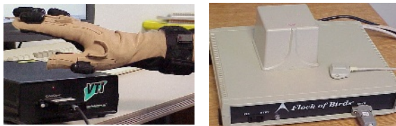
Fig. 1. The image on the right is Cyberglove™. The image on the left is Flock of birds® 3-D motion tracker
