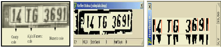
Fig. 3. A Turkish VLP on the right, horizontal projection in the middle and VLP character segmentation on the left
