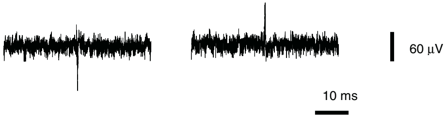
Fig. 4. Extracellular potentials recorded from the lumen a microchannel threaded by a neurite. Electrodes at different locations record spikes correlated in time but with different shapes/signs
