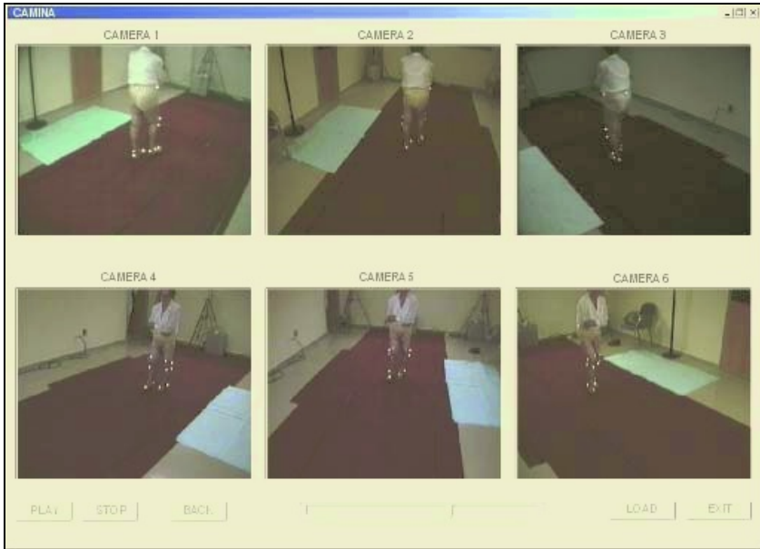
Fig. 2. Placement of markers on bony landmarks, and scenario for gait analysis, as recorded from the six cameras, where the markers are clearly identified in the image
