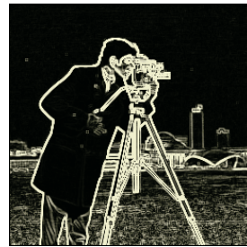
Fig. 22. Prewitt operator applied to image
