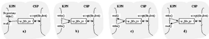
Figure 12.10. A KPN process access conditions in uc_fifo_rv border channel for deadlock study.
