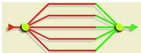
Fig. 2. The schematics of a memory with 5 channels and selection valves (the light grey circles)
