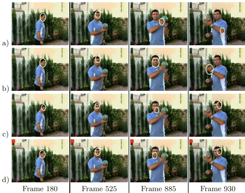
Fig. 3. Test Sequence 1, tracking with RGB histograms. a), b) and c): simple models shown in Figure 2; d): multiple model (on the upper-left corner of the images, the best model for that frame is shown).
