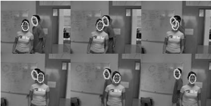
Fig. 6. Tracking multiple targets. The system is able to track multiple close target faces without confusion between them or with distracters (arms for instance). Simple face overlapping and occlusions are resolved thanks to the linear model prediction and estimation correction
