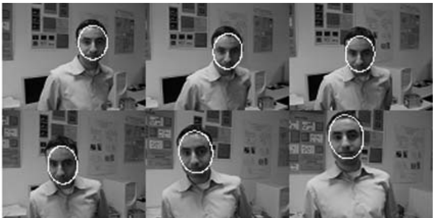
Fig. 4. The elliptical model tracks target face size and orientation as they change over time even in presence of complex target and camera movement dynamics
