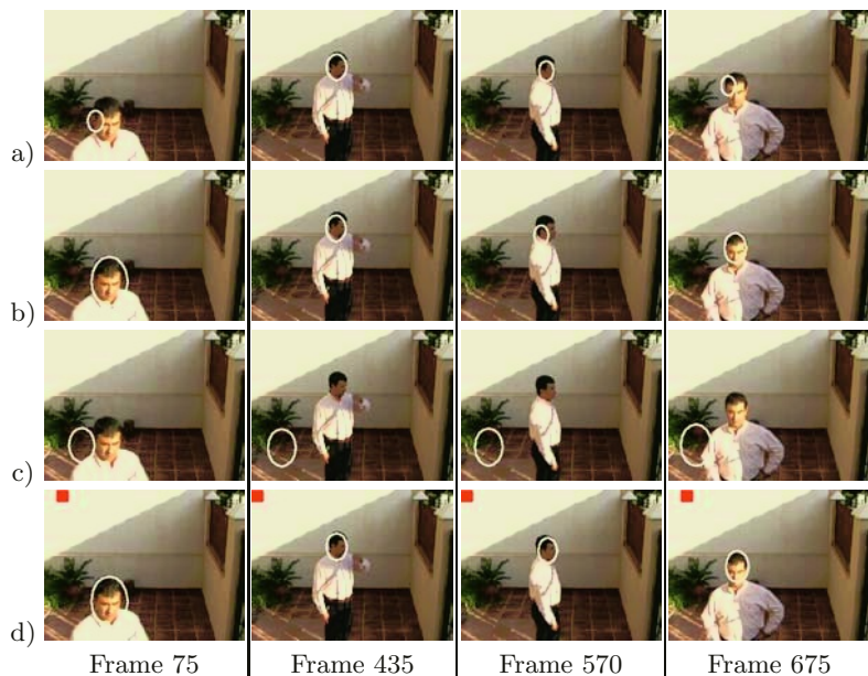
Fig. 4. Test Sequence 2, tracking with RGB histograms. a), b) and c): simple models shown in Figure 2; d): multiple model (on the upper-left corner of the images, the best model for that frame is shown).
