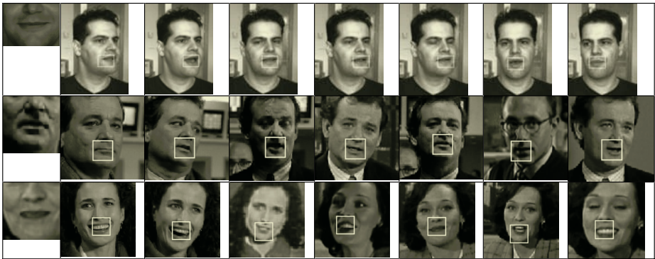
Fig. 2. This figure shows relevant results for the mouth-matching problem. In each row, the region-template used is shown in the first column. The first row shows images from a recorded sequence and the second and third row show the results from the Oxford database. The white rectangle indicates the best matching region.
