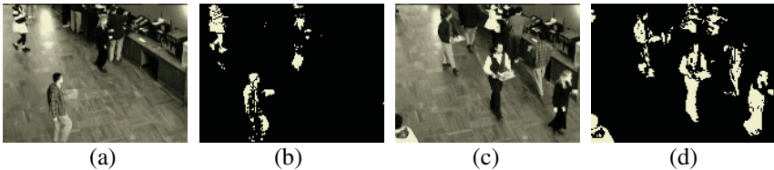
Fig. 2. Foreground segmentation in the clutter scene, (a) and (c) are the original images of the 420th and 450th frame, (b) and (d) are the segmentation result.
