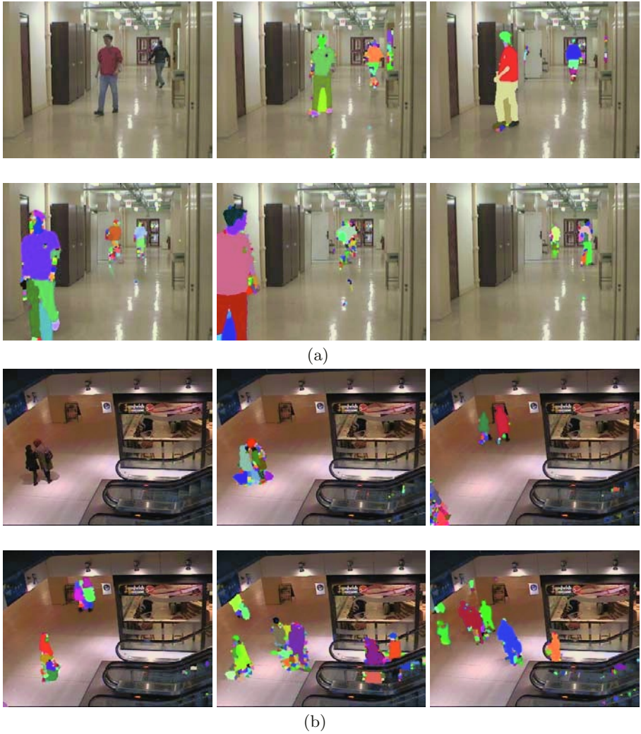
Fig. 4. From top-left to bottom-right (for each data set): first image of the sequence and moving regions detected in some subsequent frames
