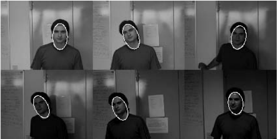
Fig. 5. Tracking in the case of severe lighting changes. Thanks to the color model update and the robustness against changes in the SPI values of the ellipse fitting algorithm, target face location and spatial extent are preserved. This video sequence shows three main different lighting conditions. The system is also able to track the target during the transitions
