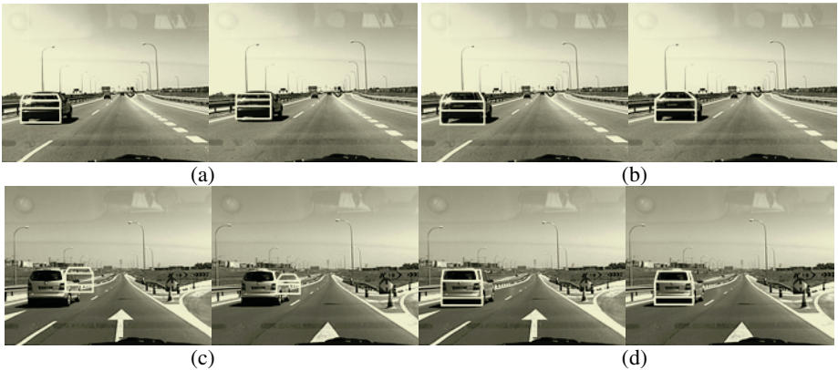
Fig. 4. Advantages of a multi-resolution approach. (a) small errors in the vehicle detection (b) multi-resolution detection (c) wrong detection (d) multi-resolution detection
