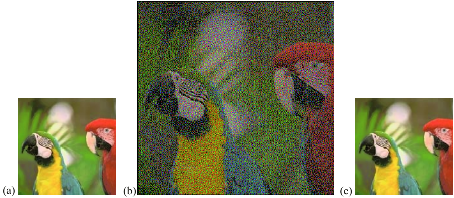
Fig. 1. Obtained results: (a) color test image Parrots, (b) the decrypted output obtained using the VSS scheme, (c) the decrypted output obtained using the bit-level processing based secret sharing scheme
