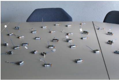
Fig. 11. Prototype implementation of Multi-SDJS on Particle Computers
