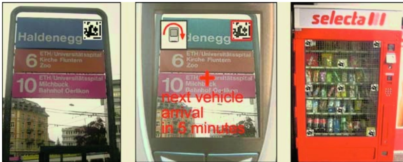
Fig. 2. A tram stop (left and middle) and a vending machine (right) equipped with visual code image maps
