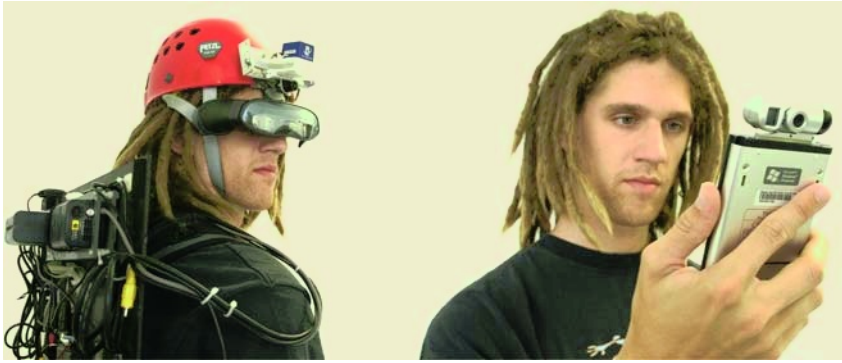
Fig. 1. A typical “backpack” setup (left) for Mobile AR versus a lightweight handheld device (right)
