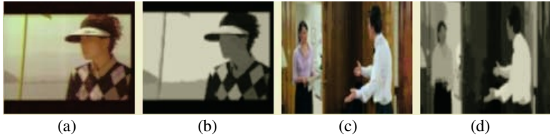
Fig. 1. Homogenous region segmentation examples: (a), (c) original images; (b), (d) their respective homogenous regions segmentation
