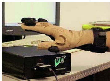
Fig. 1. Cyberglove™ with 18 sensors
