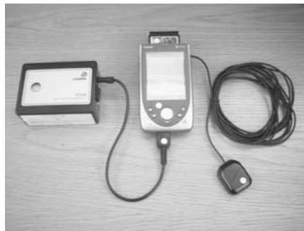
Fig. 1. The ICOM carbon monoxide sensor on the left, the PDA in the middle and the GPS aerial on the right. The HAICOM GPS unit can just be seen sticking out of the top of the PDA
