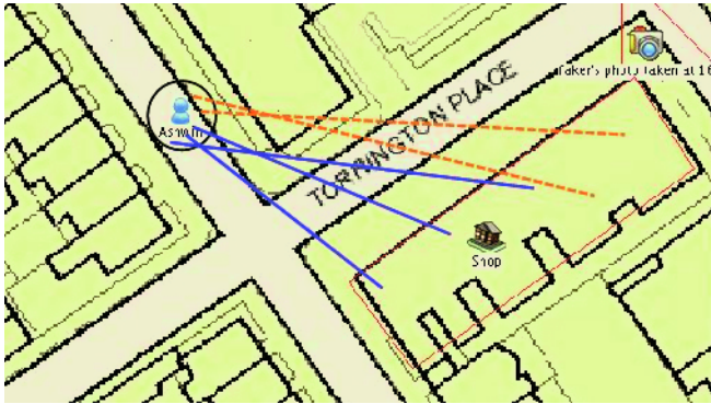
Fig. 3. Visibility computation for the filter - A random point is taken in the region around the location (the circle). Another random point is taken on the target building, and ray is defined between them. The thicker rays hit the target while the thinner rays are obstructed by buildings in their path
