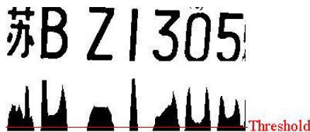
Fig. 6. Segmentation in horizontal direction
