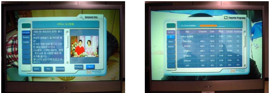
Fig. 7. Detailed Information of selected program (left) and snapshot of program list recommended by metadata service server (right)
