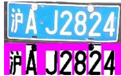
Fig. 12. Degraded top coordinate correction due to pin
