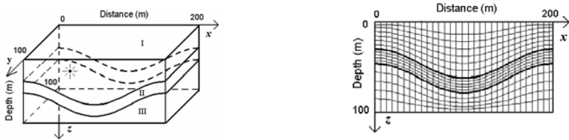
Fig. 3. (a) (left figure) 3D model with curved layer in Cartesian coordinate; (b) (right figure) Irregular grids discretization at x - z cross section
