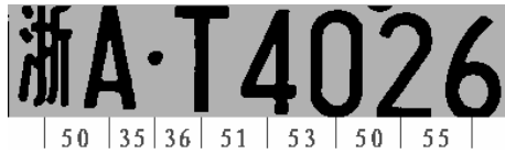
Fig. 8. Mis-segmented characters (due to space mark)
