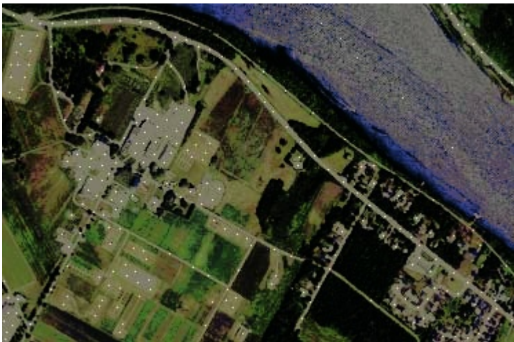
Fig. 5. Road center pixels (white) found by CLATIN algorithm (Test area 1)
