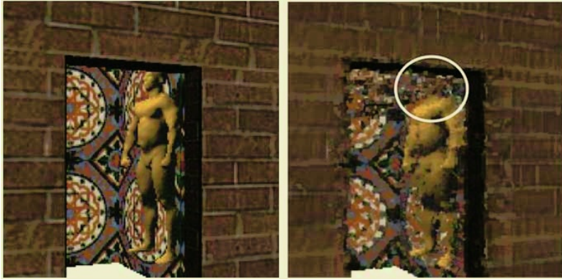
Fig. 1. Details lost by the space carving technique [6]. Left: source image, right: rendered result from the same viewpoint
