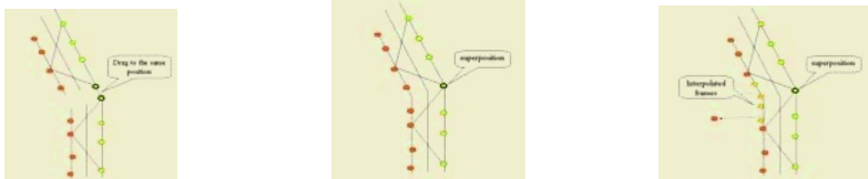
Fig. 5. footskate removal: (left) Two rearranged motion stages, (middle) drag the second motion stage to superpose the two feet, (right) remove the inter frames and interpolate transition frames
