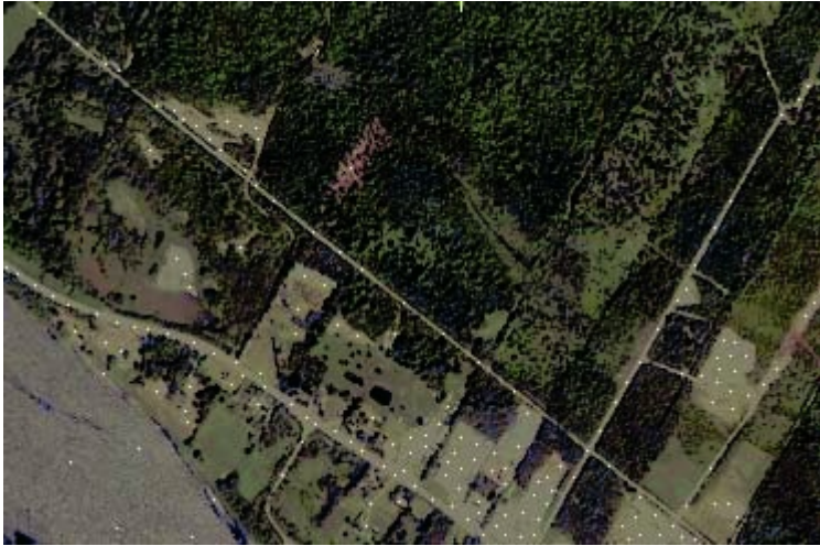
Fig. 6. Road center pixels (white) found by CLATIN algorithm (Test area 2)
