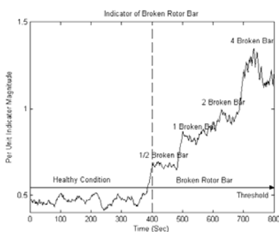
Fig. 11. Indicator of Broken Rotor Bar
