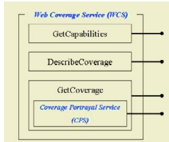
Fig. 3. Web operations, including WCS and CPS together, provide GeoTIFF and JPG data
