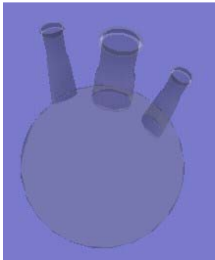
Fig. 2. A three-necked flask realized in VRML. The Java engine classifies the connections (see also Fig. 3) as FL1 (left), FL2 (middle) and FL3 (right)
