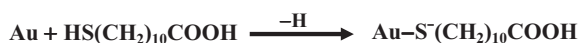
FIGURE 7.5. Thiolate formation with gold substrates: thiols react with gold surfaces by the formation of thiolates, which occurs with hydrogen loss by the sulfur atom.
