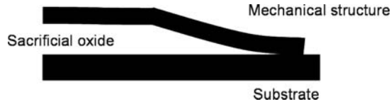
FIGURE 5.2. A small opening for sacrificial oxide etching that will release a mechanical structure.
