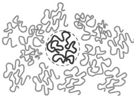
Fig. 17 Schematic illustration of a single polymer chain contracted in a two-dimensional monolayer. Reprinted with permission of [26], copyright (2003) The Chemical Society of Japan
