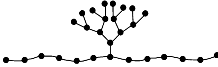
Fig. 21 Polymer chain bearing a dendritic wedge in its middle
