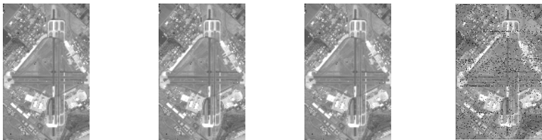
(a) JPEG quality 100% (b) JPEG quality 80% (c) JPEG quality 60% (d) JPEG quality 40%
