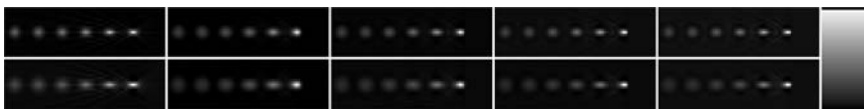
FIGURE 12. Efficacy of iterative CDRF compensation for LEHR (top row) and LEGP (bottom row) collimators. The images shown are transaxial images from reconstructions of projections of the phantom shown in Fig. 7. They have been truncated to the region of the point sources. The leftmost source is located at the center of rotation. The columns were reconstructed using (left to right) FBP and OSEM with 64 subsets per iteration at 5, 10, 20, and 30 iterations, respectively.
