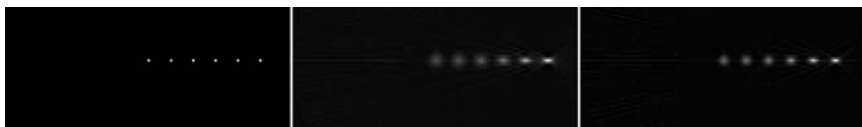
FIGURE 7. Effect of the GRF on SPECT image resolution. The image on the left is a point-source phantom. The middle and right images were reconstructed using FBP from projections obtained using LEGP and LEHR collimators, respectively. The image has been truncated at the top and bottom.
