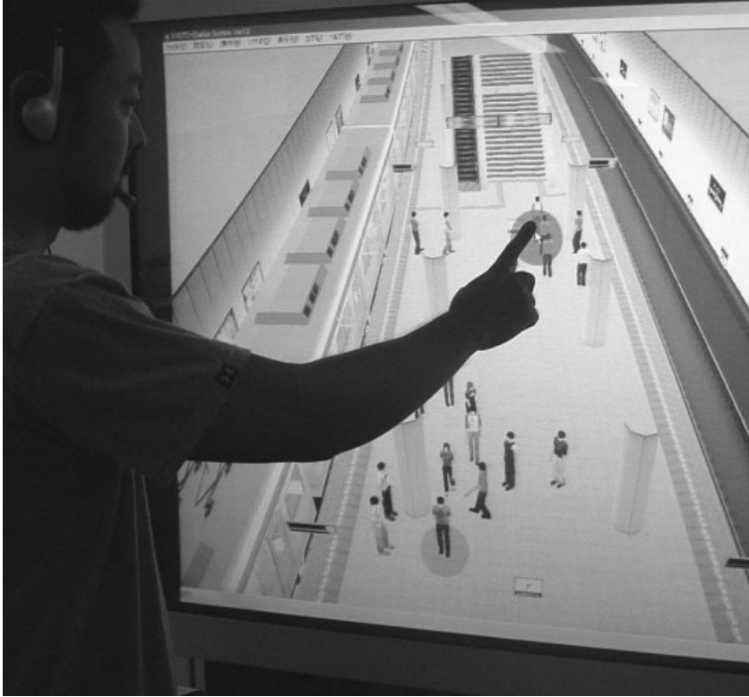
Fig. 4. Evacuation guidance system
