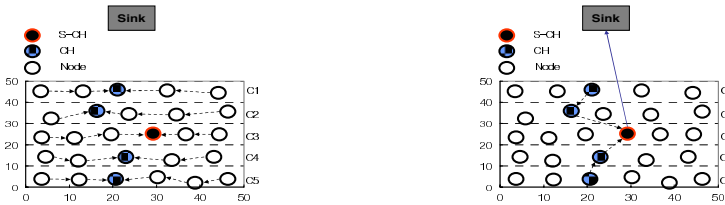
(c). Data gathering in each cluster (d). After data gathering from each CH to the SCH, the SCH sends all information to the sink
