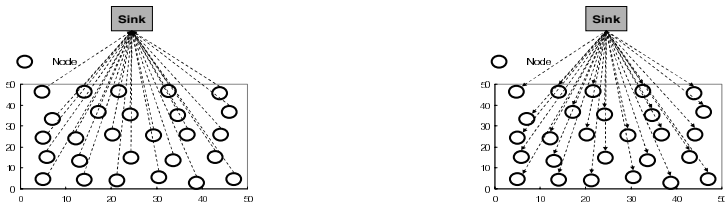
(a). All nodes send their information to the sink (b). The sink sends cluster information to nodes
