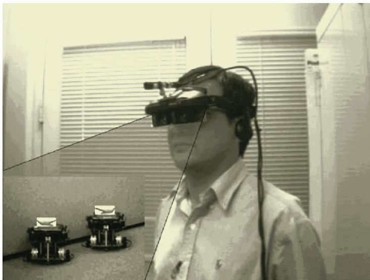
Fig. 6. Coded infrared signals are decoded into arrows for overlay onto a real scene. These are visible via the augmented reality head-mounted display system with camera.
