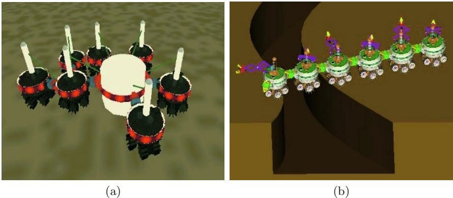
Fig. 1. Graphic visualisation of how the rigid gripper can be used to connect in a secure way s-bots among themselves so that they form a swarm-bot for (a) retrieving heavy objects or (b) passing over holes.
