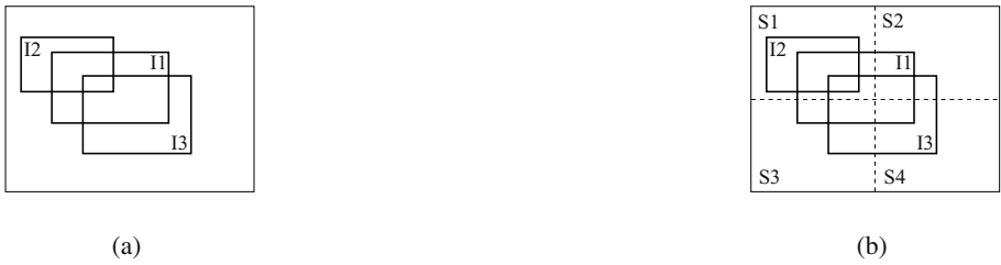
Fig. 4. Screen-parallel compositing. Dividing the screen into subscreens produces more parallelism of image compositing
