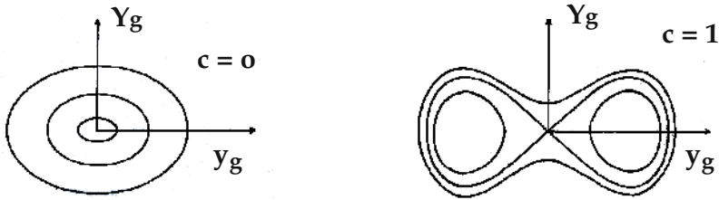
Fig. 7. Motion of the particle around its gyrocenter for the Hamiltonian (63) with F = 2 , k = 1 , Y_c = 0 and two particular values of c .
