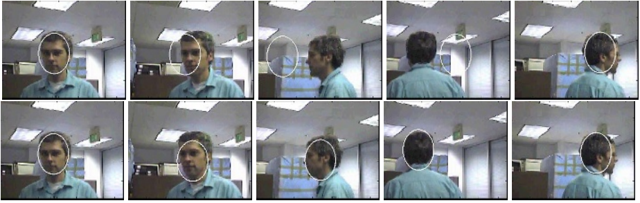
Fig. 4. Tracking results with the conventional PF (top) and the UAPF (bottom). From left to right, the frame numbers are 3, 18, 31, 40 and 50. From frame 18 on, the motion of the tracked object moves towards the inverse direction of the pre-assumed motion direction which makes the conventional PF lose the target. In contrast, the UAPF can track the whole image sequence successfully
