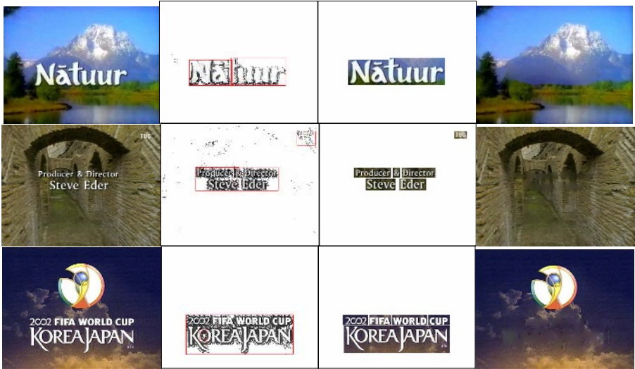
Fig. 5. Example of caption detection and removal. Test frames (first), detected caption regions (second), and segmented caption region (third), and removed caption frame (last)
