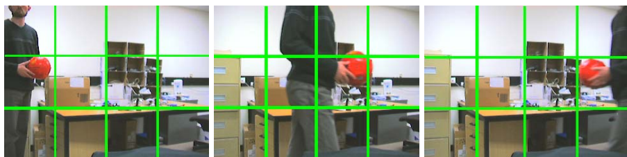
Fig. 1. Training the Markov model. Each 80 by 80 pixel square is assigned a state. Each transition of the red ball between states (the image regions bordered by grid lines, shown here in green) is recorded
