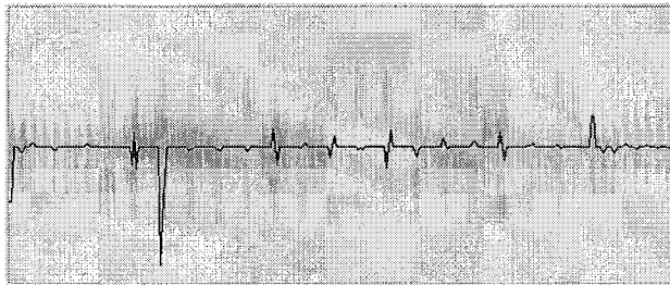
Zoomed view of the usage of second input byte and the power trace (gray)
