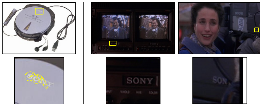
Fig. 2. Object query example II: searching for a Sony logo. First column: (top) Sony Discman image with the query region outlined in yellow and (bottom) close-up with detected elliptical regions superimposed. Second and third column: (top) frames from two different shots of ‘Groundhog Day’ with detected Sony logo outlined in yellow and (bottom) close-up of the image. The retrieved shots were ranked 1 and 4 (from 8 retrieved in total).
