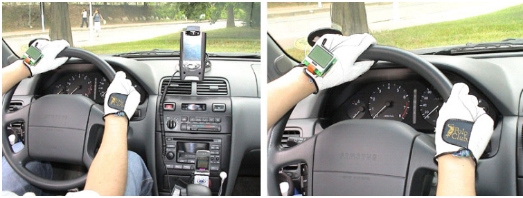
Fig. 3. A glove-based Wearable Multimedia Interface for wireless control of a navigation system on an iPAQ PDA and in-vehicle multimedia systems
