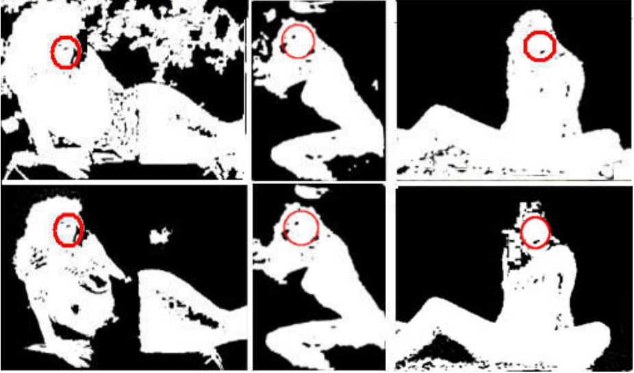
Fig. 3. Skin detection result. The top row are coarse skin detection results, the bottom row are the final refined results. For offensive reasons, original images are not presented here.
