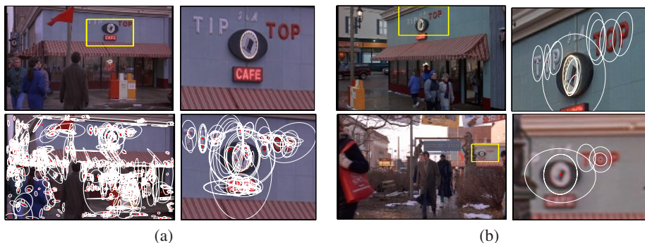
Fig. 1. Object query example I. (a) Top row: (left) a frame from the movie ‘Groundhog Day’ with a query region in yellow and (right) a close-up of the query region delineating the object of interest. Bottom row: (left) all 1039 detected affine co-variant regions superimposed and (right) close-up of the query region. (b) (left) two retrieved frames with detected region of interest in yellow and (right) a close-up of the images with affine co-variant regions superimposed. These regions match to a subset of the regions shown in (a). Note the significant change in foreshortening and scale between the query image of the object, and the object in the retrieved frames. Querying all the 5,640 keyframes of the entire movie took 0.36 seconds on a 2GHz Pentium.
