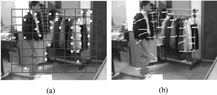
Fig. 2. Block-based Motion Estimation (a) the selected 9x9 region for block motion estimation (b) the extracted block vectors
