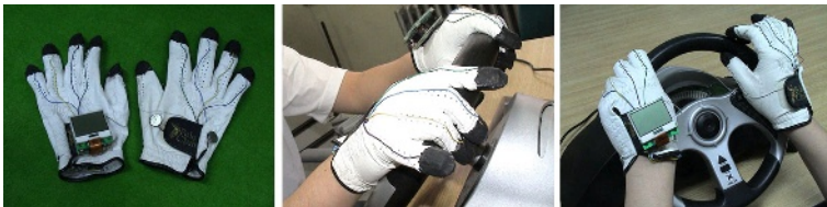
Fig. 2. The wearable multimedia interface (WMI) developed (left), and finger motions for making input using the WMI. Input can be made by simple tapping or by chording using two or more fingertips at the same time (center). Information of control mode and functions activated are shown on a small LCD of the left hand(right)
