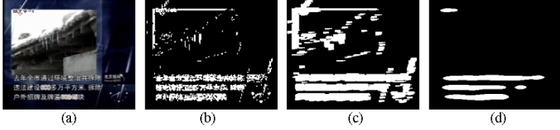
Fig. 3. (a) Original image, (b) Candidate pixels, (c) Candidate text regions by morphological “close” operation and (d) by “density-based” region grow.
