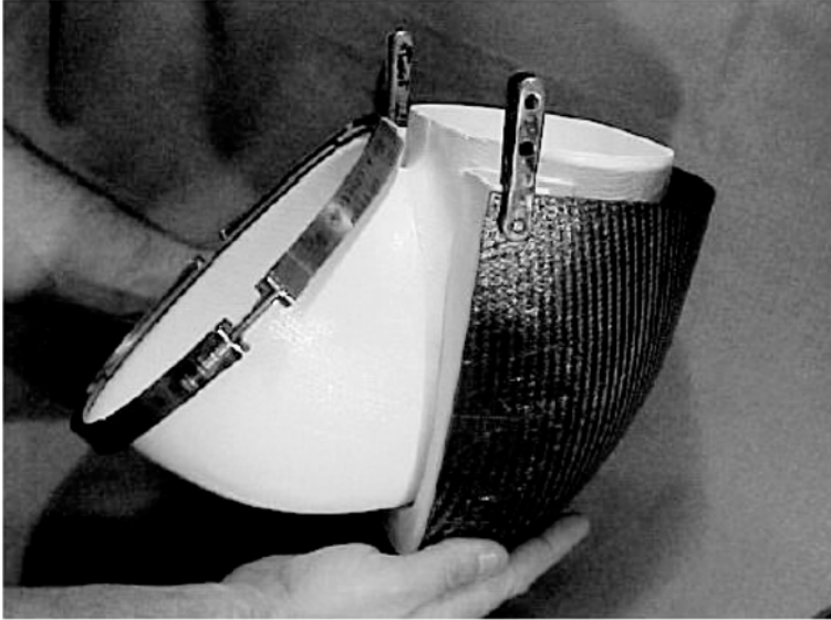
FIGURE 1. A lightweight helicopter exhaust duct for insulating and protecting the surrounding structure. (Courtesy COI Composites Inc., Materials Research and Design, Inc., & U.S. Navy)
