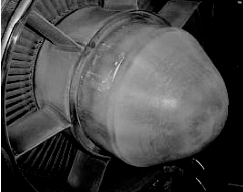
FIGURE 22. SiOC Nextel 312 BN Tailcone Installed for Allison Engine Test (after 1500 hour test exposure)
