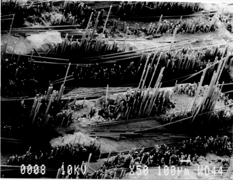
FIGURE 31. Nextel™ 610/Al 2 O 3 composite fracture surface following tensile testing at room temperature.
