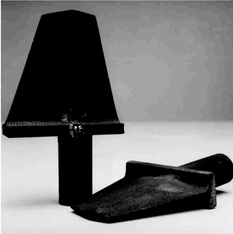
FIGURE 3. C/C-SiC jet vanes for solid fuel rocket propulsion systems
