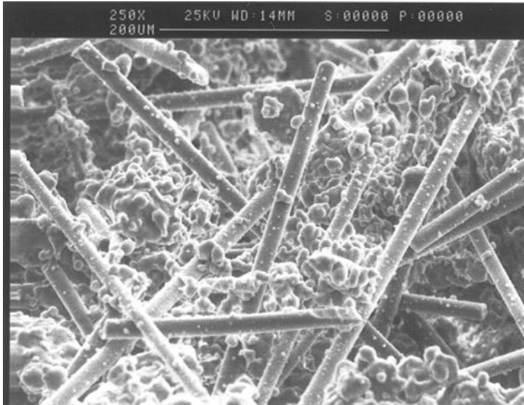
FIGURE 3. Microstructure of a SiC chopped fibre reinforced glass matrix composite showing the fairly homogeneous mixture of the composite constituents attained by wet-mixing.
