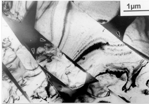
FIGURE 4. TEM micrograph of the microstructure of a glass/alumina In-Ceram composite showing no microcracking development at the interface between the glass (dark) and alumina (light) phases [16]. (Photo courtesy of Dr. H. Hornberger).
