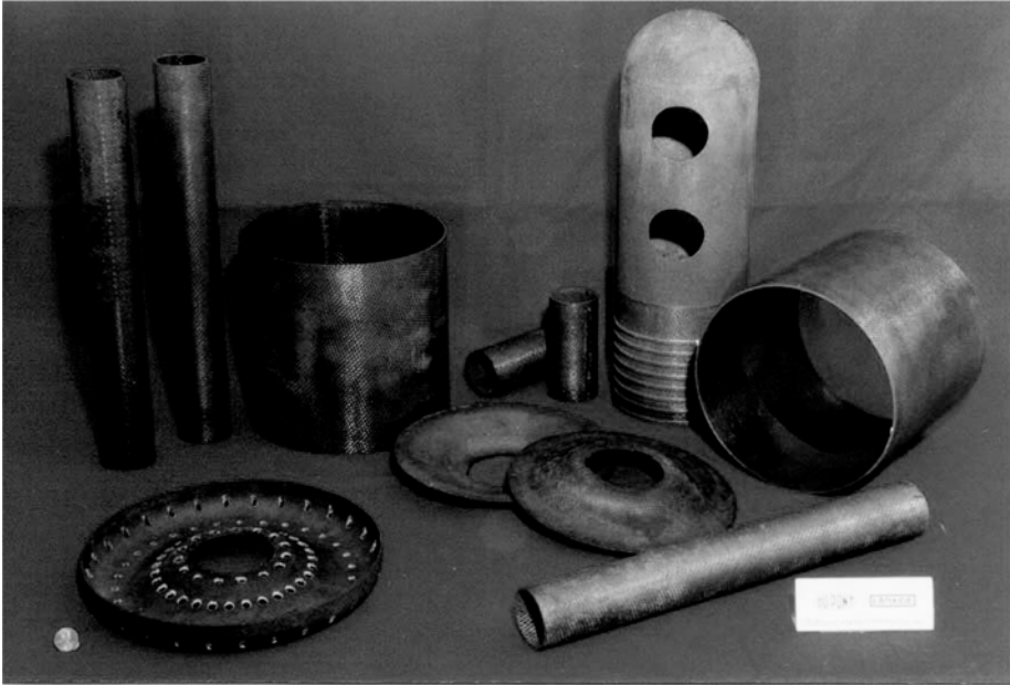
FIGURE 19. Nicalon TM /Al 2 O 3 components fabricated using the directed metal oxidation process.
