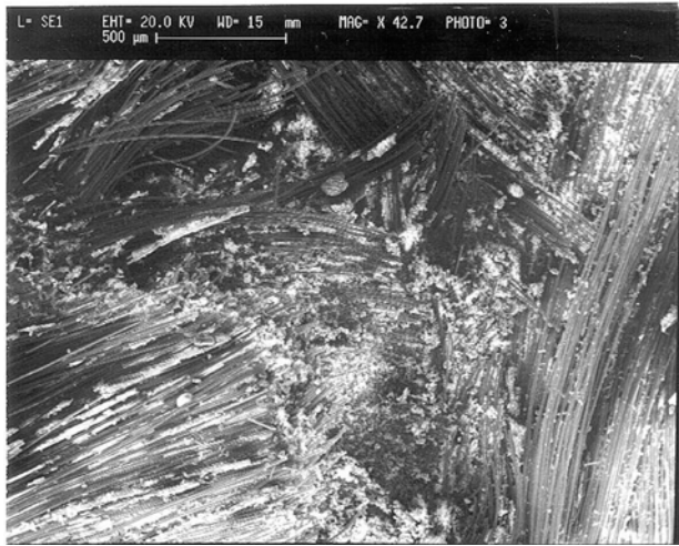
FIGURE 2. SEM image of the fracture surface of 3-D Tyranno ® fibre-reinforced aluminosilicate glass matrix composite tested in compression [10].
