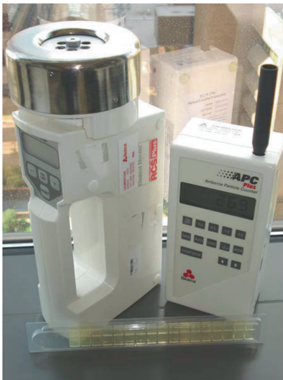
Fig. 13.1 Electronic counters. Left: Viable counter with agar strip shown at the base. This strip is inserted into the drum-shaped chamber at the top of the counter and viable organisms are deposited onto the strip during monitoring. Right: Particle counter
