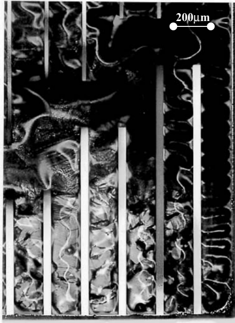
Fig. 24. Array of PZT/SOI microcantilevers. Backside view before the final release—etching of the buried SiO 2 .
