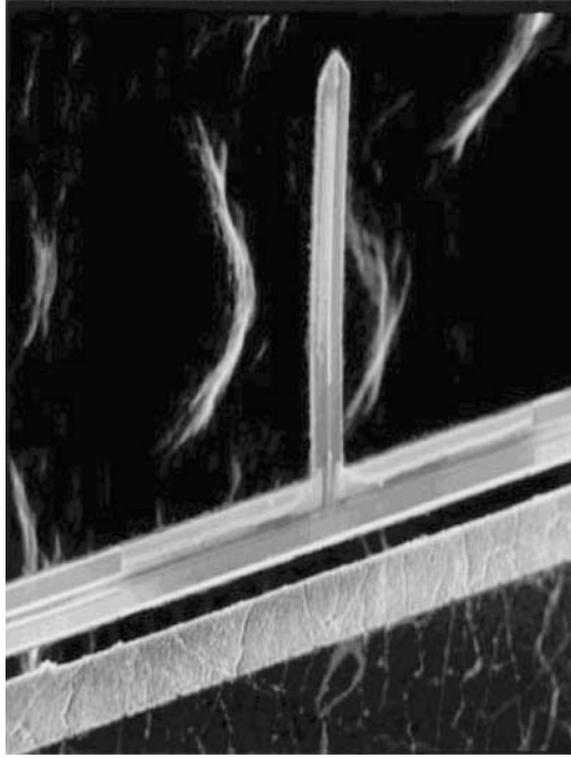
Fig. 2. Fabricated AFM cantilever with XYZ actuation by PZT thin film layer.
