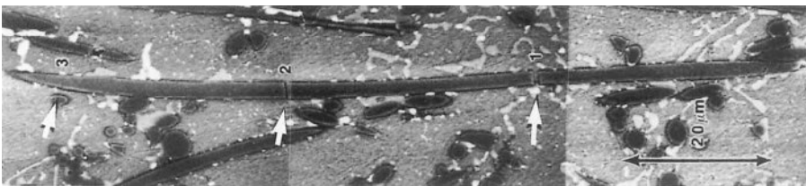
Fig. 9.11 Fiber fracture (indicated by arrows) in \text{Al}_2\text{O}_3 short fiber reinforced \text{Al}_7\text{Si}_3\text{Cu} alloy matrix composite during creep (courtesy of A. Dlouhy and G. Eggeler). The loading axis is horizontal.
