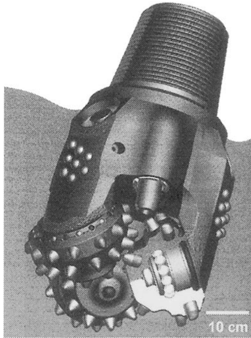
Fig. 11.30 Roller cone bit used for oil well drilling. The rock cutting inserts are made of WC/Co metal matrix composites. (Courtesy of A. Griffo, Smith International, Inc.)
