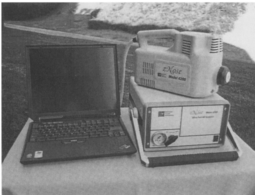
Figure 1. The zNose™ Model 4200 Analyzer, Photo courtesy of Electronic Sensor Technology
