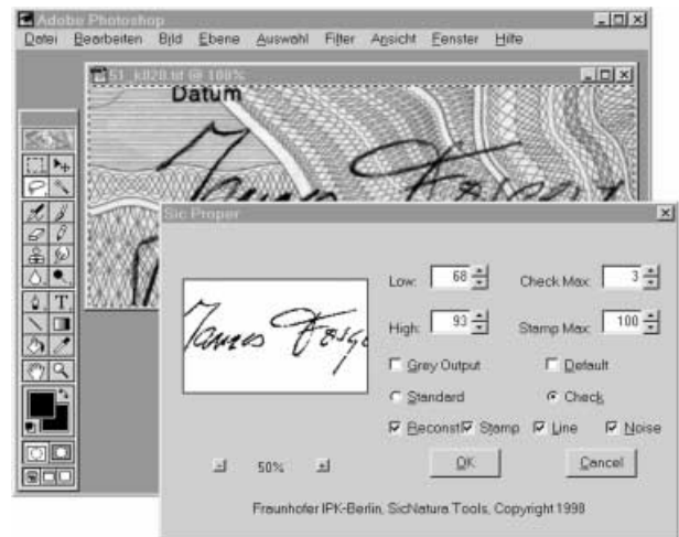
Fig. 5. Specific methods, taking into account the typicality of handwriting, realized as Plug-In for Adobe Photoshop
