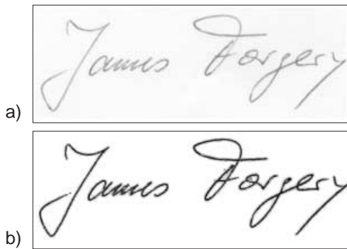
Fig. 11a,b. Local contrast enhancement: a) original signature image; b) signature image after processing
