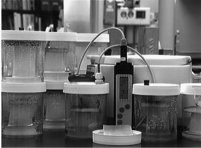
Fig. 1. Moisture chambers with wallboard samples.
