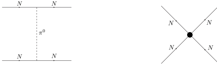
Figure 2. CP-odd nucleon-nucleon processes which induce nuclear level CP-odd moments. The left diagram is the long range nuclear force. It is generated by combining the CP-even and the CP-odd pion-nucleon interactions. The upper (lower) vertex represents the CP-even (CP-odd) interaction. The right figure depicts the CP-odd contact nucleon-nucleon interaction.
