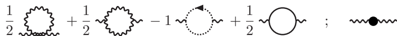
Figure 1. The self-energy diagrams contributing to order \ell^1 . Wiggly/dotted/full lines denote gluons/ghosts/scalars, respectively. In the notation of eq. (5.5), the first four diagrams give \Pi_T^{(1),0} , while the last is \Pi_T^{(0),1} .
