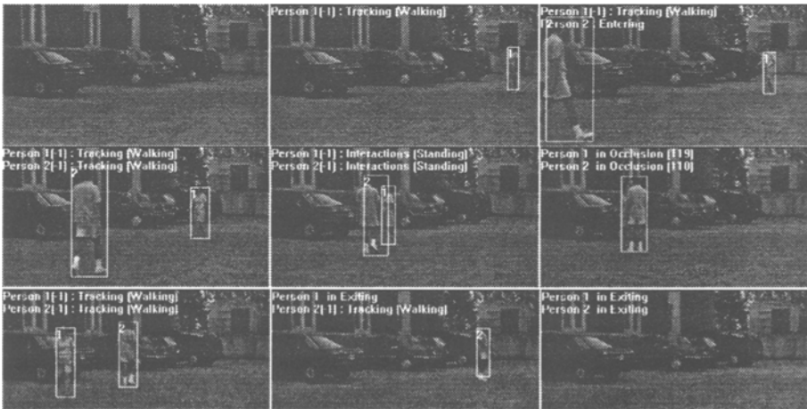
Fig. 9. An example for W^4S tracking; two people are entering, walking, meeting and leaving
