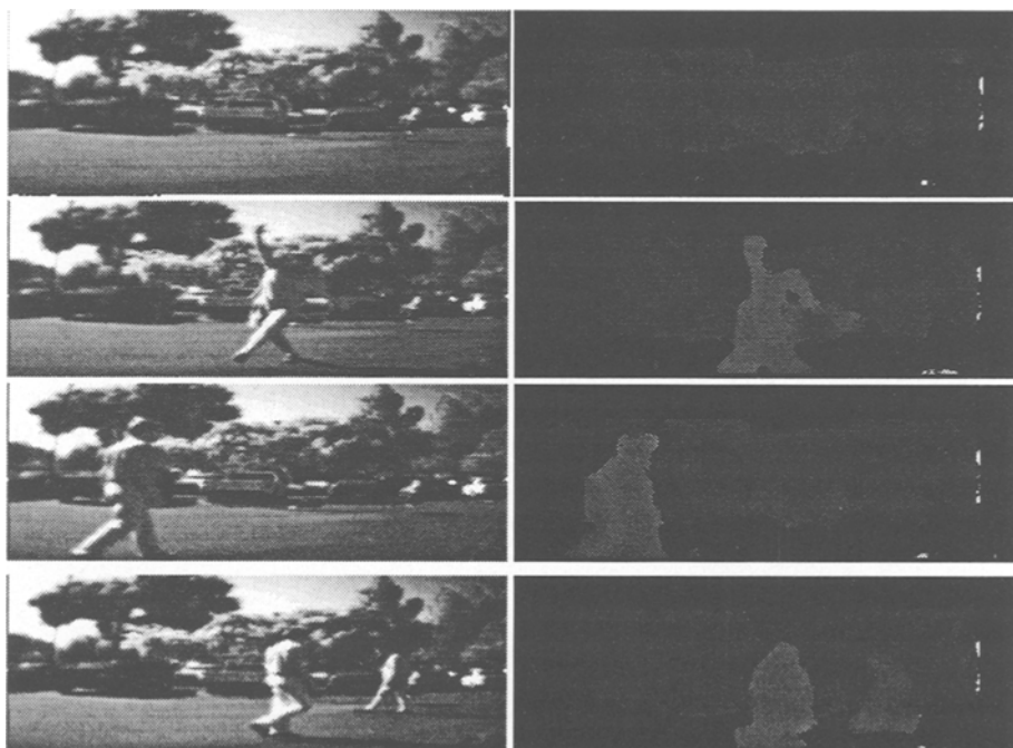
Fig. 3. Examples of the range images calculated by area correlation stereo
