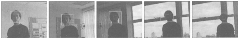
Fig. 6. Five frames from a sequence in which a face was tracked using a non-adaptive model. The apparent colour of the face changes due to (i) varying illumination and (ii) the camera's auto-iris mechanism which adjusts to the bright exterior light.
