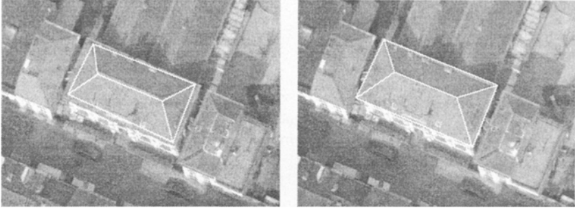
Fig. 6. Left: Back-projecting the roof model of Fig. 5 into the original images illustrates the loss of metric accuracy during the 3D grouping and roof modelling process. Right: Metric accuracy can be restored by changing the wireframe model so as to minimize the reprojection error in all the available images.
