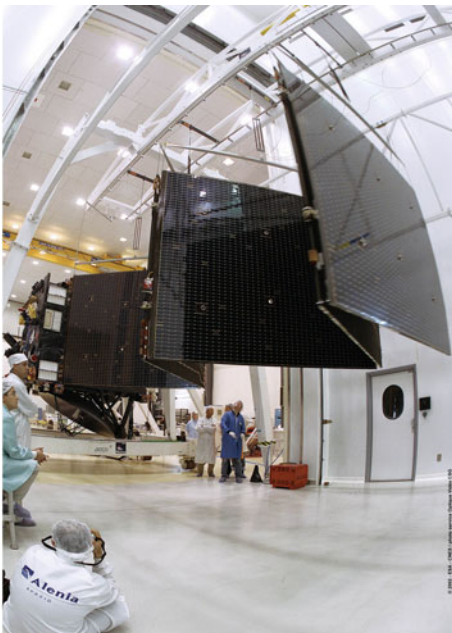
Figure 4. Rosetta solar panels during a deployment test (credits: ESA/CNES)
