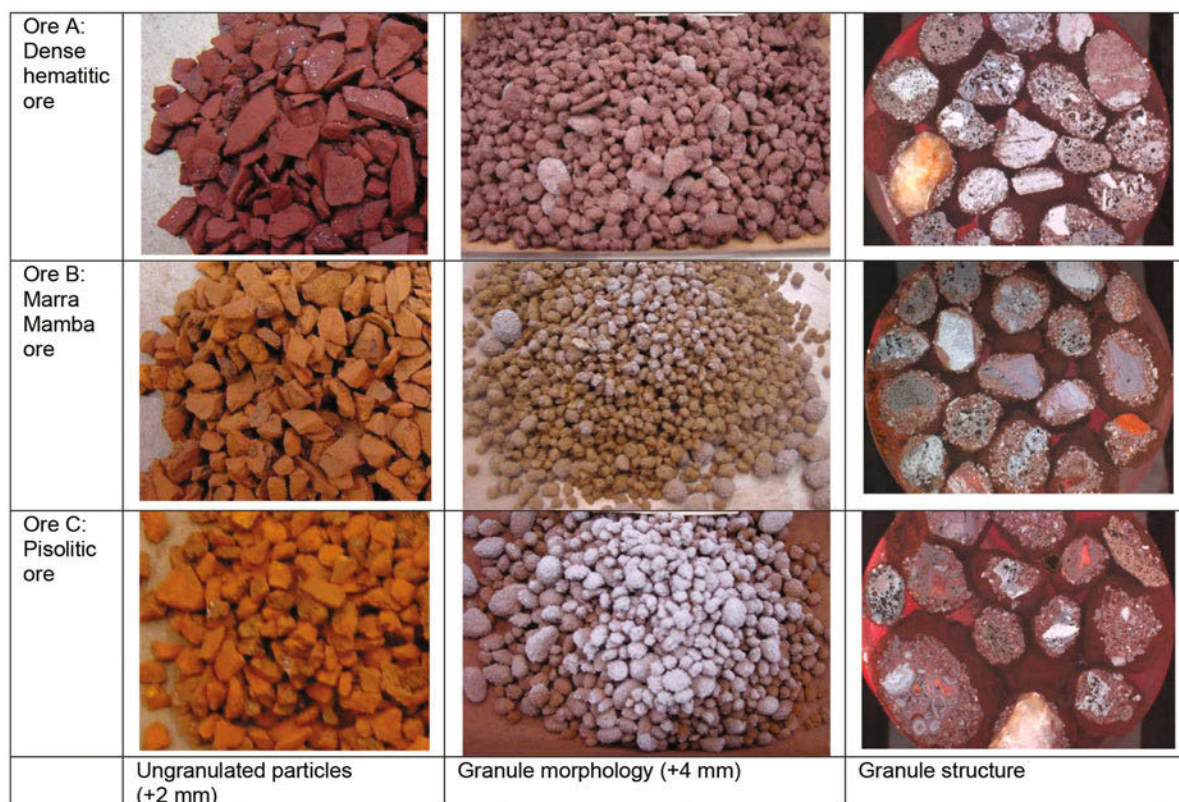
Figure 9 — Effect of particle shape and surface morphology on the morphology and structure of the green granules.
