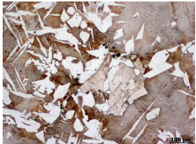
Figure 17. Micrograph of 1030 with 0.2% RS sample.
