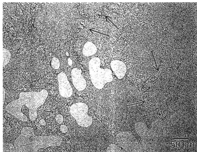
Figure 16. Distribution of \beta Phase in an Al-10%Si alloy (56) (Arrows show \beta plates located at eutectic grain boundaries).
