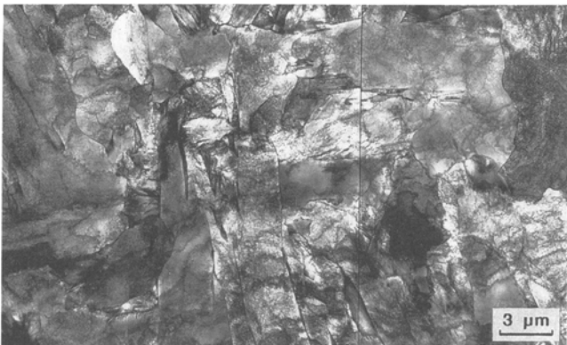
Fig. 10—Transmission electron micrograph of the simulated ICRCG HAZ which consists of upper bainite, martensite, and ferrite.
