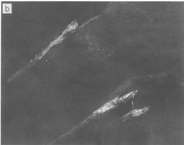
Fig. 12—(a) Bright-field and (b) dark-field transmission electron micrographs of the simulated ICRCG HAZ, clearly showing the typical dislocated martensite with interlath retained austenite.
