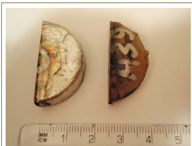
Figure 2 – Picture of the upper and lower half-button surfaces once the sample has been cut in order to start the metallographic preparation procedure of its transverse cross-section
