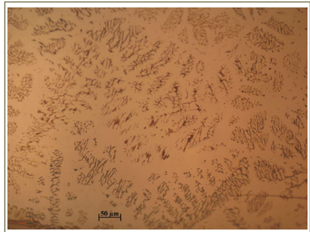
Figure 9 – Lathy ferrite morphology in [FA] Sample A32 ( Cr_{eq}/Ni_{eq} = 1.46 , [Cr_{eq} + Ni_{eq}] = 40 wt%)
